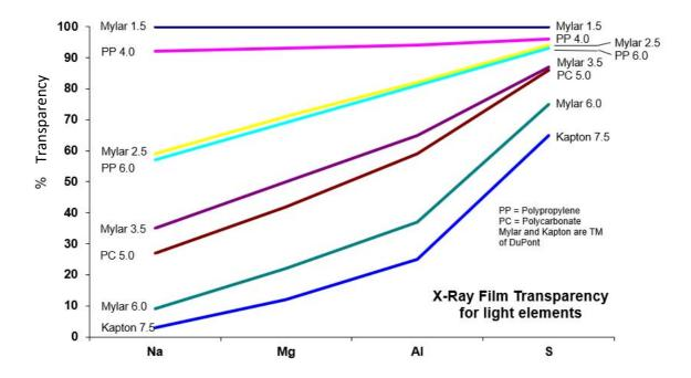
**Polypropylene** is especially suited to the trace analysis of solid samples, as it has no major contamination in it. In contrast, **Mylar** contains the undesirable phosphorus and calcium (3.5  $\mu$ m Mylar corresponds to 50 ppm Ca and 250 ppm P in a straight oil, e.g., clean white oil).
